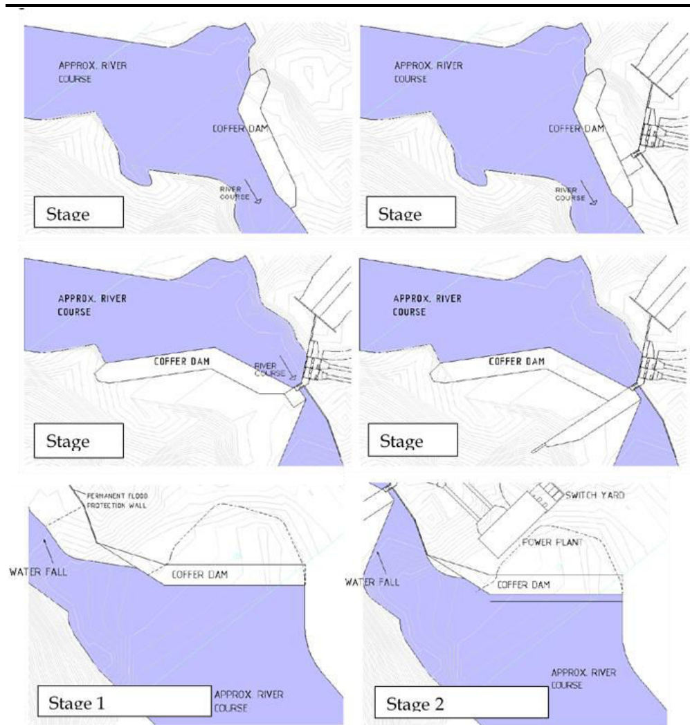
Figure 3.11 Stages of River Diversion for the Construction of the Hydropower Plant
